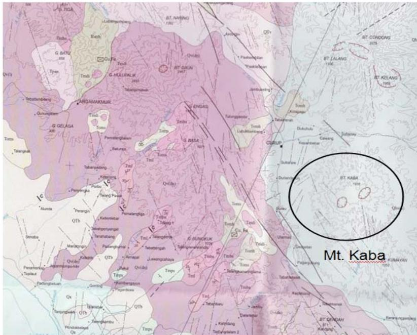
**Figure 2.** A geologic map of surrounding area of Mt. Kaba (scale 1:100,000). Circle indicates the location of Bukit Kaba, the highest peak at Mt. Kaba. Qhv: quaternary breccias; Qvi: quaternary andesitic-basalt; QTV: quaternary andesitic; Tomh: tertiary lava; Tmba: tertiary breccias.
