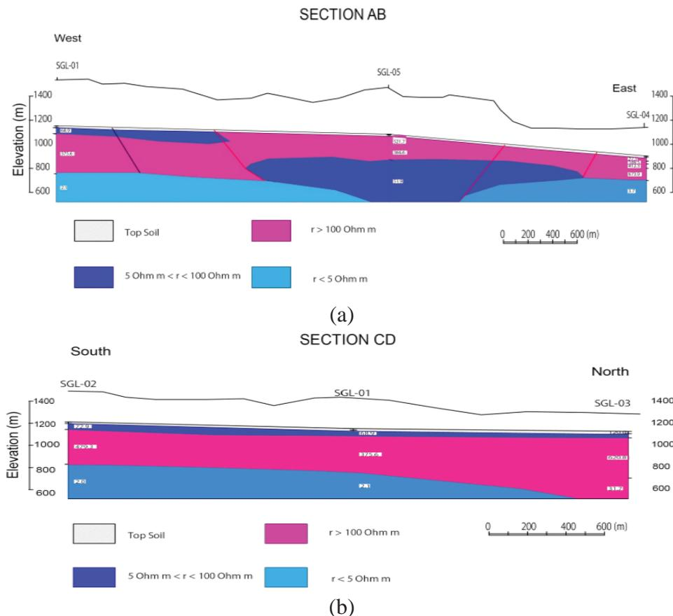
**Figure 6.** True resistivity observed at sections (a) AB and (b) CD. Low resistivity less than 5 ohm-m is observed at about 400 m depth from the surface.
