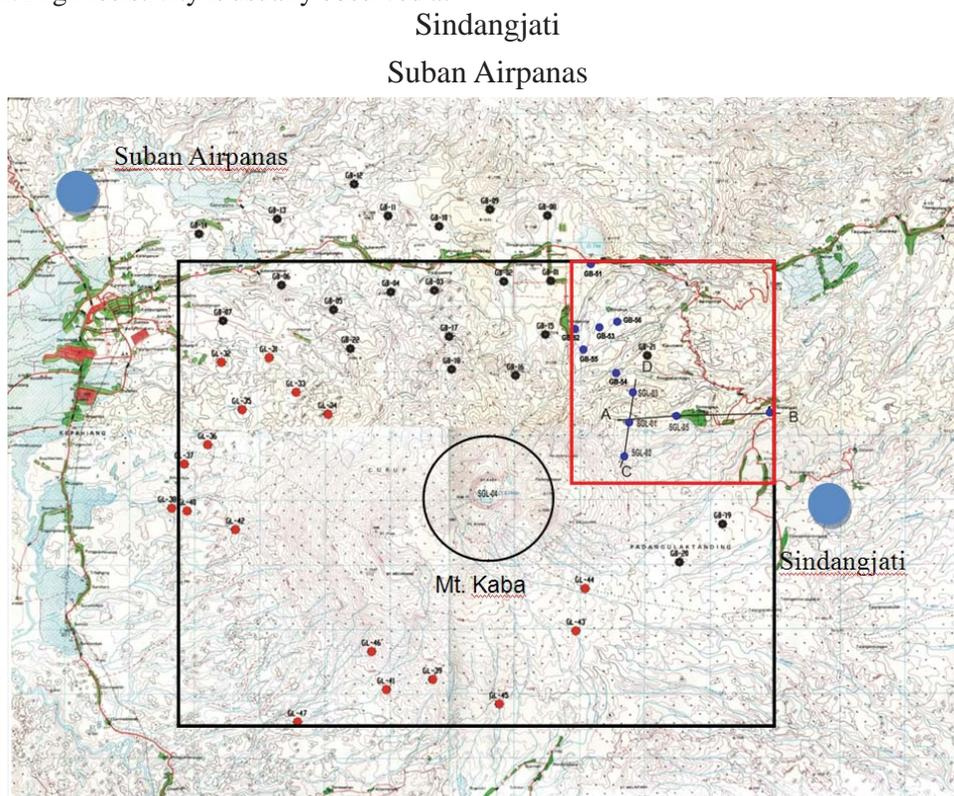
**Figure 3.** Locations of geoelectrical survey surrounding of Mt. Kaba (scale 1:100,000). Solid black, red, and blue circles represent the locations of the survey conducted in 2009, 2010, and 2011, respectively. Two traverses lines AB and CD are also shown. Black square indicates the area used for resistivity contour with AB/2 1,200 m. Red square indicates the area used for resistivity contour with AB/2 1,600 m and 2,000 m.
