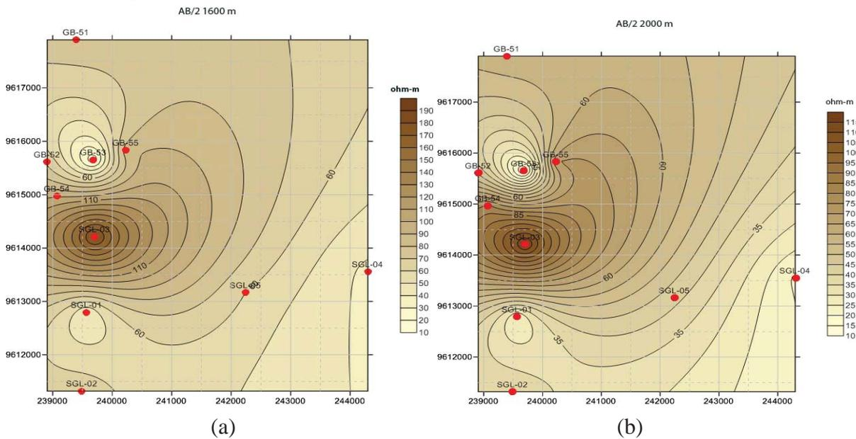
Figure 5. Spatial distribution of apparent resistivity at AB/2 (a) 1,600 m and (b) 2,000 m.
