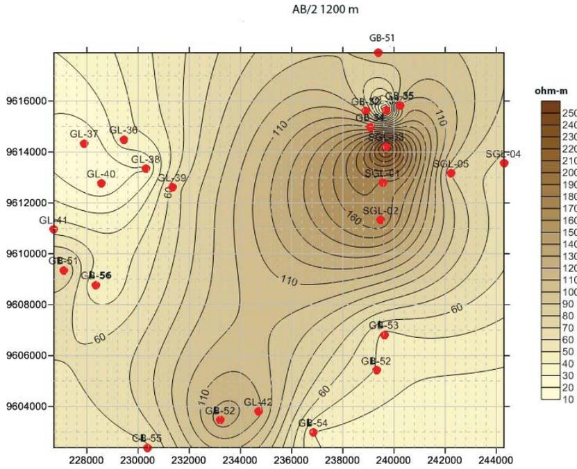
Figure 4. Spatial distribution of apparent resistivity at AB/2 1,200 m.
